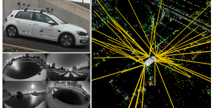
Fig. 1. We aim at accurately localizing the UP-Drive vehicle depicted in the upper-left corner in a map of visual features depicted on the right side. Features are extracted from images of the surround-view camera system (lower-left corner) and matched against 3D landmarks in the map. Inlier matches, centered on the estimated 6DoF pose of the vehicle in the map, are illustrated as dark yellow lines on the right side.
